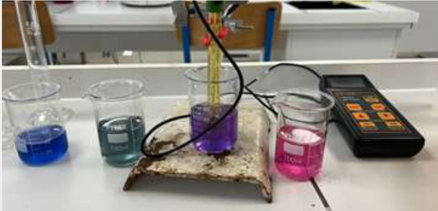
Measuring the pH of our samples with a pH meter
