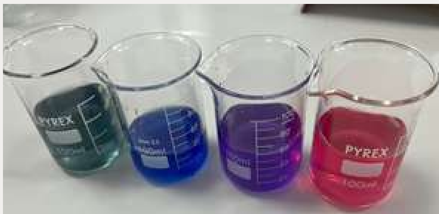
Beakers with samples of clitoria infusion with different pH (resp 12.3-5.8-3-1.7)
